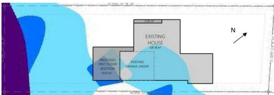
Figure 1: GIS flood map overlay on the owners’ property and the proposed building work (purple = overland flow path, dark blue = inundation/ponding depths > 300mm, light blue = inundation/ponding depths 100-300mm)
