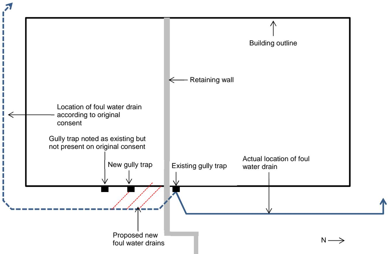
**Figure 1: Diagram of proposed and existing drainage system (not to scale)**
