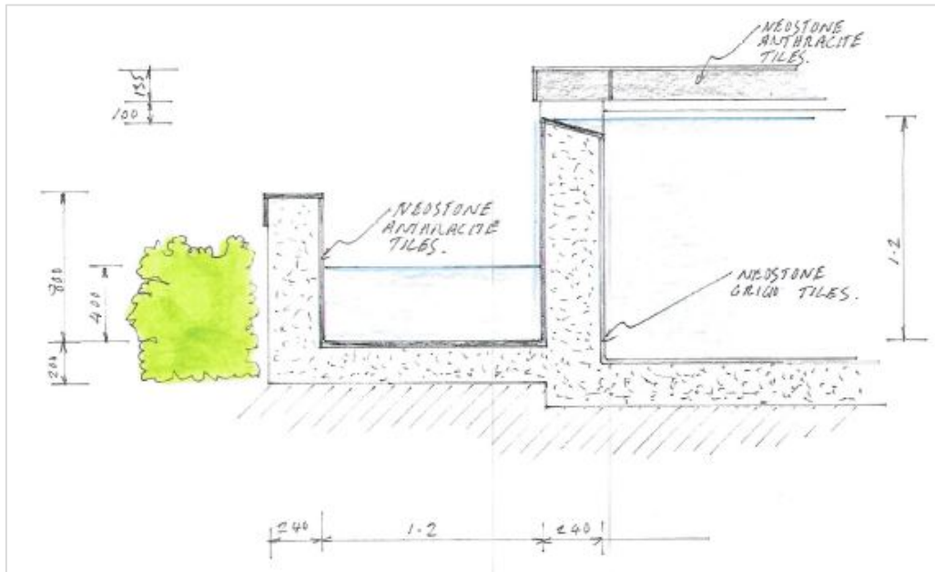
Figure 2: Balance tank and infinity edge as designed – detail of consented plans
