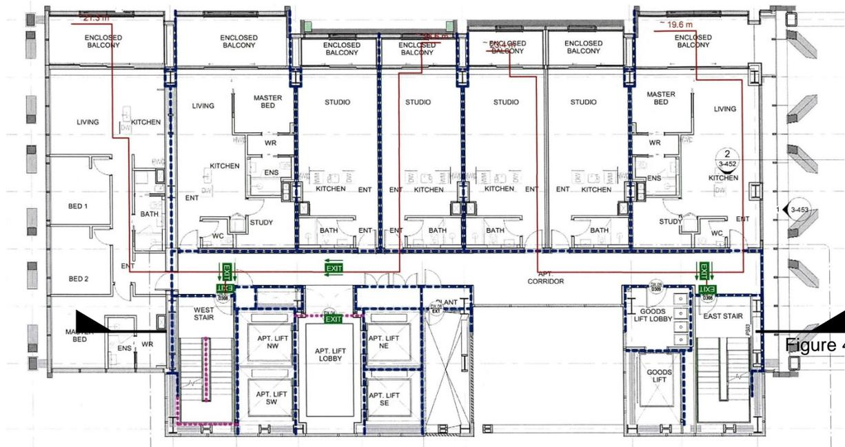
**Figure 3(b): Plan L40 showing transition corridors from Upper West Stair (not to scale)**
