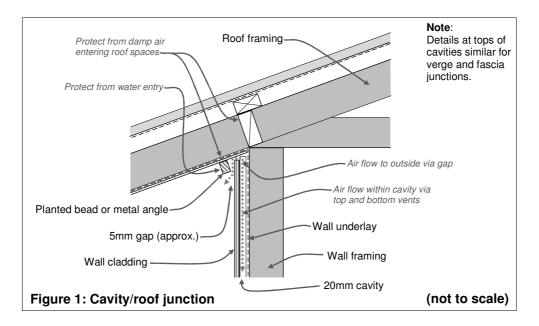
2.3.2 The junction provides ventilation within the cavity by way of a gap of about 5mm at the top to allow air flow to the outside, while protecting the junction from water penetration with the use of planted beads or metal angles. The roof and eave framing is intended to be sealed from damp air with blocking and wall underlay.
