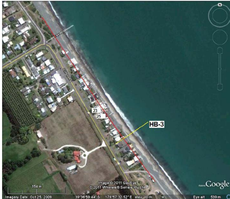
Figure 1: Vertical aerial photograph showing the location of Nos 23 & 25 Clifton Road and HBRC Beach Profile HB-3. The red line marks the erosion scarp or landward limit of the beach, seaward of which lies active dynamic beach subject to wave action.
