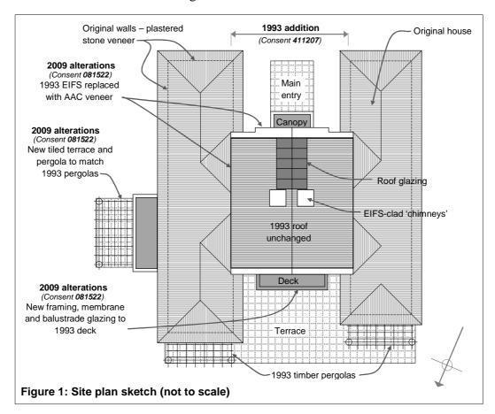
2.2 Construction is generally conventional light timber frame, with concrete foundation walls, suspended timber floors, plastered masonry veneer to original retained walls, AAC veneer to additions, profiled metal roofing and aluminium windows. The altered house is fairly complex in plan and form and is assessed as having a high weathertightness risk (refer paragraph 7.2.2).
