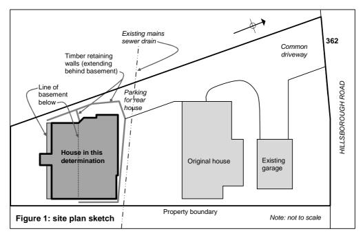
2.1.2 The un-subdivided south-sloping section narrows towards the rear where it is 'benched' with timber retaining walls to provide two building platforms. One of these walls extends through the subfloor of the house, while the other borders the west, north and east sides of the building platform. An existing mains sewer drain crosses the section; and is shown on the site plan as 1 metre north of the upper retaining wall.
