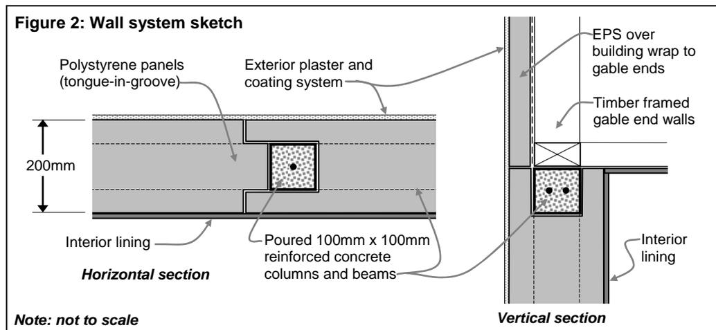
3.3.2 The main walls of the house are constructed from 200mm thick interlocking polystyrene (“EPS”) panels, which provide formwork for a reinforced concrete post and beam structure. Steel reinforcing rods connect the poured columns and beams to the foundations, the first floor framing and the roof framing. At joinery openings, timber sub-frames fit within the panel grooves, with planted solid timber packers against which the windows and door are face-fixed.
