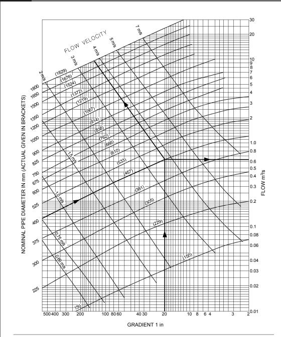
**Example:** A 450 internal diameter pipe with a gradient of 1 in 20 will have a flow of 0.63 m³/s at a velocity of 3.75 m/s
