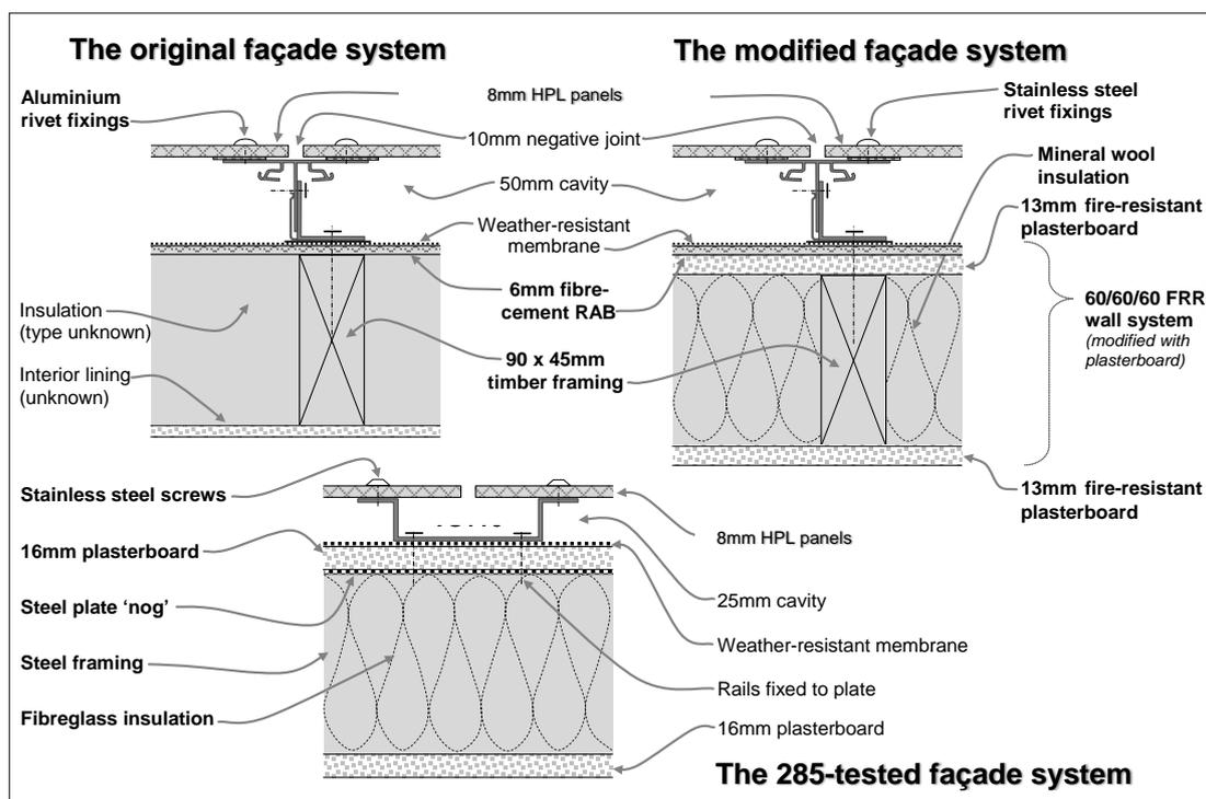
2.5.2 Components of the façade systems shown in Figure 2 are compared in Table 2:
