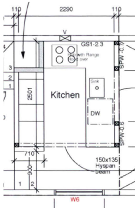
Figure 2. Detail from approved consent plans showing the location of the hob with rangehood and vent.
