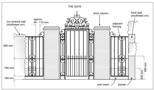
Figure 2: Sketch of gate and adjacent sections of barrier (not to scale)
