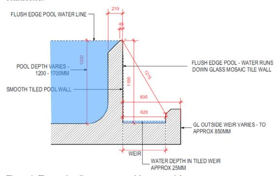
Figure 2: The pool wall as constructed (not to scale)
