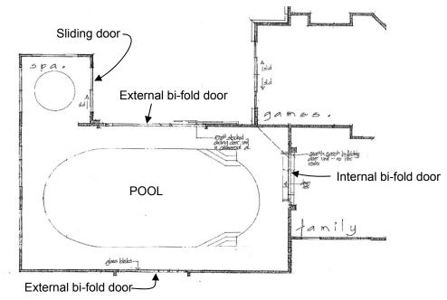
Figure 1: Plan indicating type and location of pool room doors<sup>5</sup>
