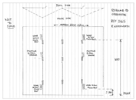
Figure 3: The internal bi-fold door<sup>9</sup> (sketch by applicant, not to scale)
