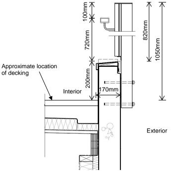
Figure 1: The proposed barrier design (not to scale)
