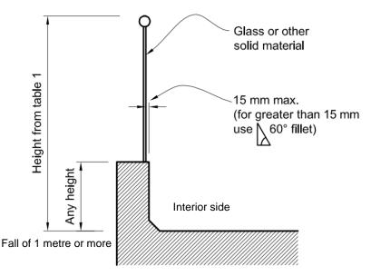
Figure 3: F4/AS1 barrier (Figure 3) – Barriers in areas likely to be frequented by children under 6 years of age – glass or other solid material
