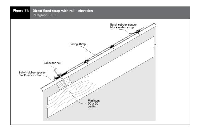
6.3.2 Solar col ors mounted on the hof cladding mus the nate als me requirement ed n Pa agraph 6.3.3 Solar collectors fixed directly to meta roof *cladding* must be:
