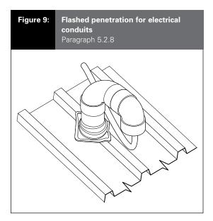
The diameter of the conduit should be the minimum practicable diameter to suit the cable size and any electrical regulatory requirements.
