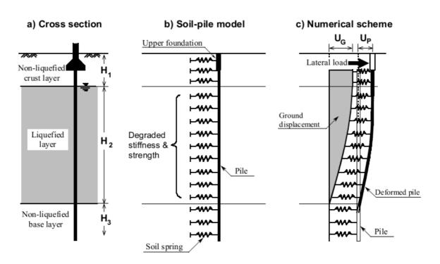
Figure 1. Pseudo-static analysis procedure for piles with lateral spreading. [Source: Cubrinovski et.al. 2009].
