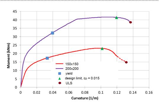
Figure 3. Example moment-curvature<sup>3</sup> relationship for small pre-stressed concrete piles (with 100 KN axial load).
