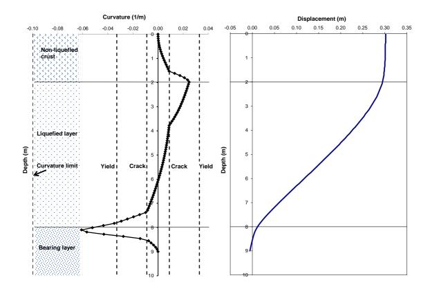
Figure 4. Curvature and displacement versus depth for 150x150 pre-stressed concrete pile at a site with 6m thick liquefied layer.
