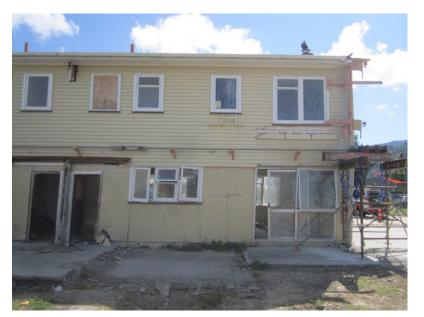
Figure C9A.2: Longitudinal test of Housing New Zealand unit showing significant racking of ground floor walls
