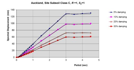
Figure C3.2: Displacement spectra for different damping levels and site subsoil class C and including appropriate near fault factor
