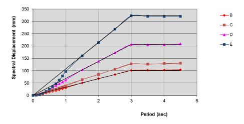
Figure C3.1: Displacement spectra at 5% damping for R = 1,  $S_p = 1$  for various site subsoil classes and including appropriate near fault factor
