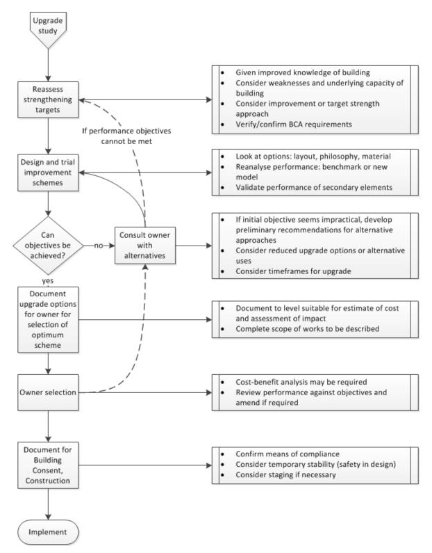
Figure A10.1: Generalised seismic upgrade process flow
