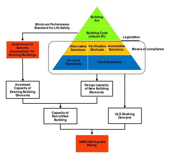
Figure A5.1: Use of Guidelines and Building Code to determine *%NBS* earthquake rating for alterations involving new building elements
