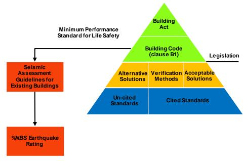
Figure A3.1: Relationship between Clause B1 of the Building Code and Earthquake Rating
