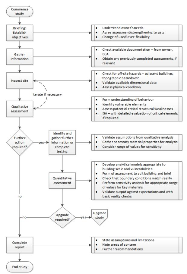
Figure A7.1: Generalised assessment process flow
