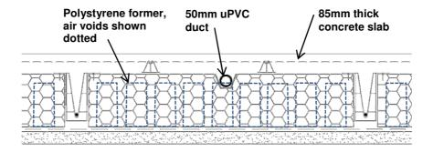
Figure 2: Schematic section showing 50mm duct located in floor slab
