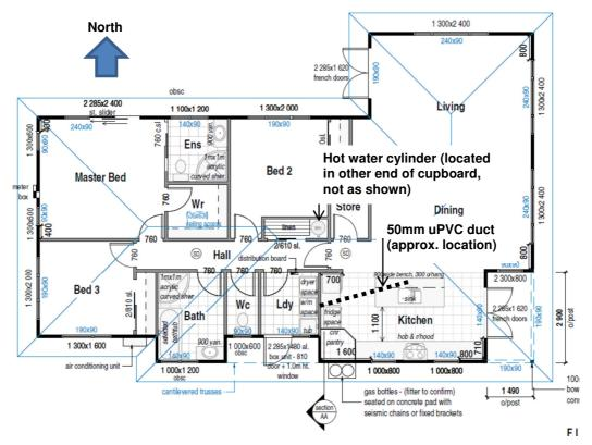
Figure 1: Floor plan of the house showing location of the duct
