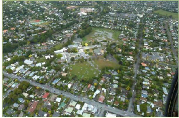
Aerial photo of liquefaction ejecta at Cashmere High School
